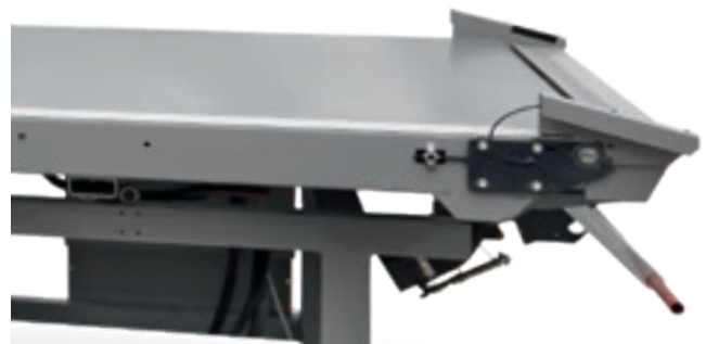
Intake manifold positioned at the end of the belt.
