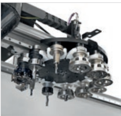
Revolver magazine with 12 overhead positions and 16 on the X carriage.
