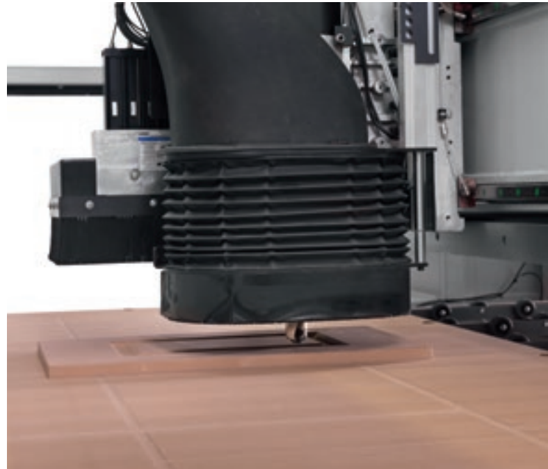
Suction hood with 12 programmable positions and the use of a continuous cover for optimum suction capacity.
